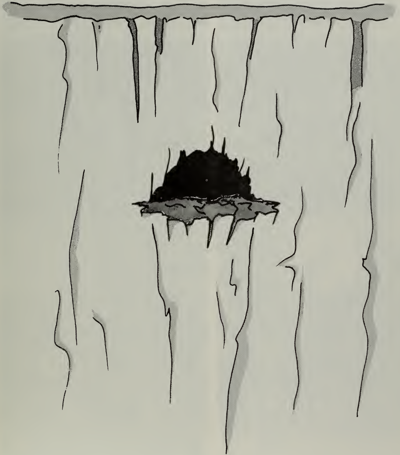
Figure 1. Artist's concept of artificial cavity that could be constructed for golden eagles, red-tailed hawks, or prairie falcons. For golden eagles, cavity or ledge should be approximately 6' long x 6' high (if a cavity) x 4' deep. Prairie falcon cavities should be about 24" long x 12" high x 16" deep.
